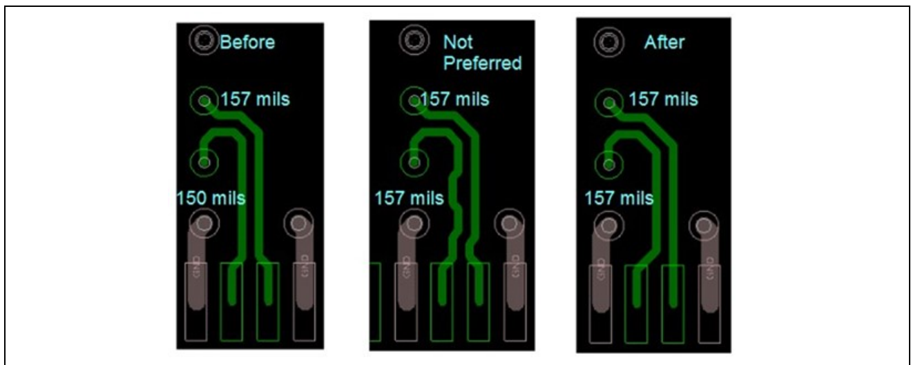
Figure 3-4. AAC connector escape routing example
